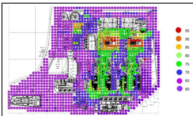
Figure 2 Noise Contour Mapping in power plant process (Spot Map)
