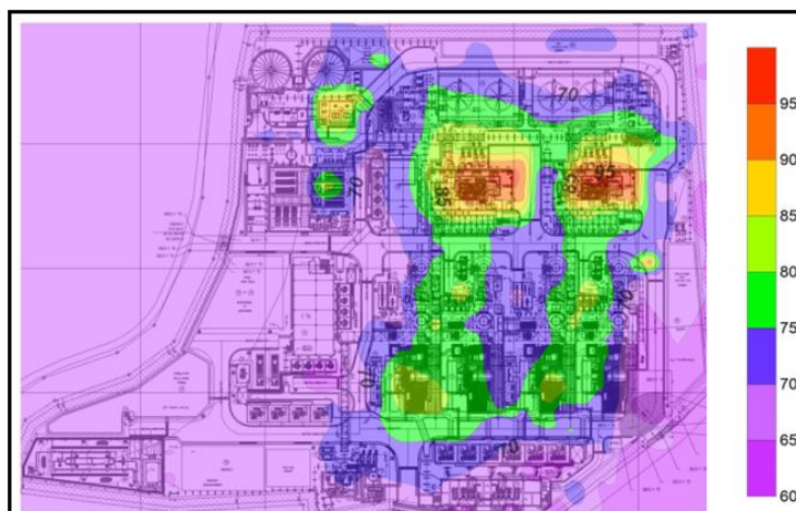
Figure 1 Noise Contour Mapping in power plant process
