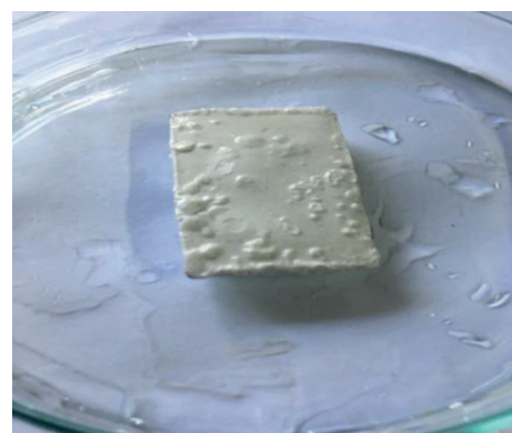
Figure 8 Artificial skull parts after immersion testing
