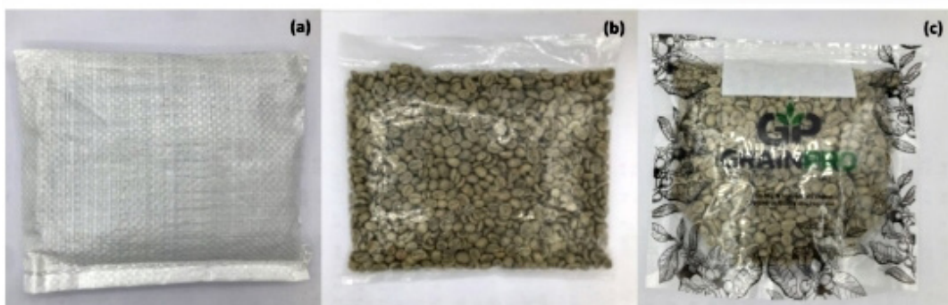
Packages for GCB storage (a) plastic woven bag (PW), (b) low-density polyethylene bag (LDPE) and (c) GrainPro® (GP).
