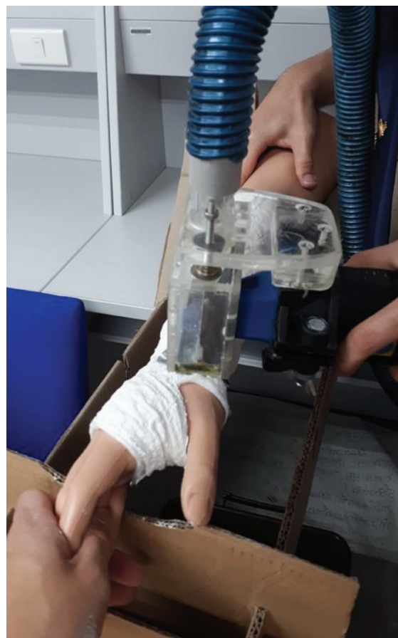
Figure 3 The use of a dust collector amalgamated with an oscillating saw and a vacuum cleaner
